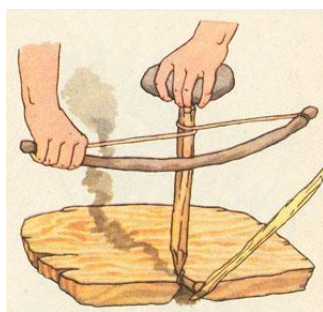
Fig. 4. Obtaining fire by friction using THREE things – a stick, a bow and a board
